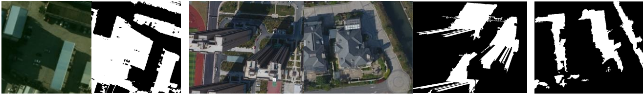
Fig.5. The result of DSDNet work. The white part is the shadow pixels. The black part is non shadow pixels
