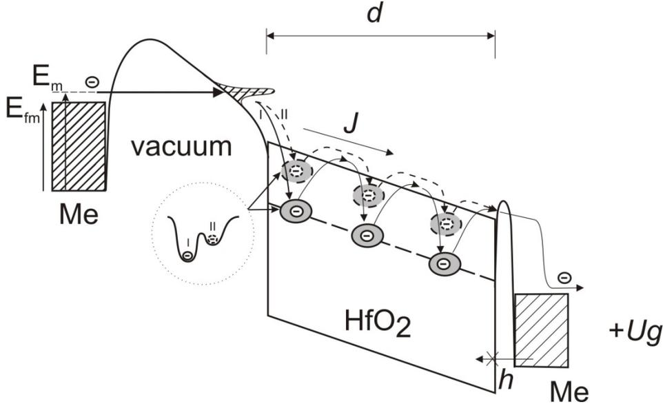
**Fig. 2.** Energy diagram of breakdown channel in hafnium dioxide with vacuum gap
