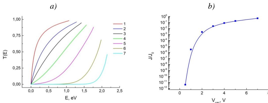
**Fig. 3.** Field emission coefficient of cathode in the hafnium dioxide breakdown channel as the function of a tunneling electron energy and the external field magnitude  $F$  (a).
