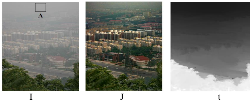
Figure 1 – Variables in the haze imaging equation. The transmission map t is shown as white when t=1 , and black when t=0 .
