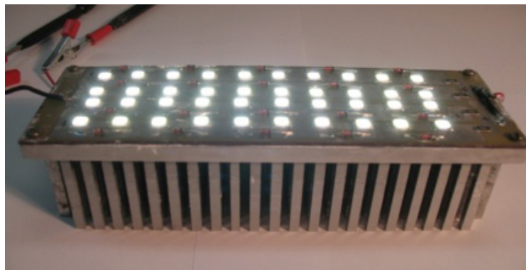
Figure 1 – High-brightness LED system on the anodized aluminum heat sink
