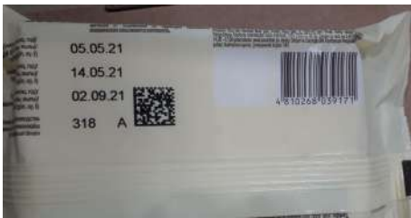
Figure 2. Product with Data Matrix code
