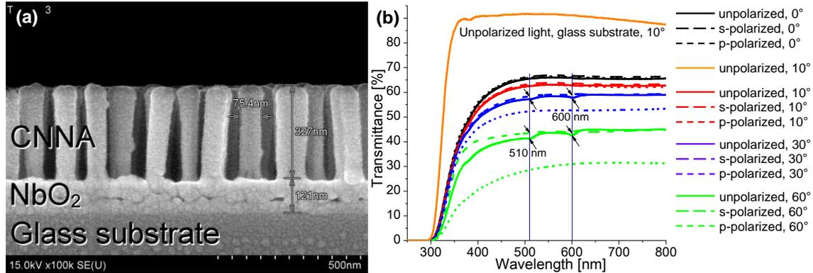
**Figure 1** Columnar nanoscale niobia array SEM-image (a) and transmittance optical characteristics (b) of glass substrate (incident angle 10°) and columnar nanoscale niobia arrays (incident angles 0, 10, 30 and 60°) formed via anodizing Al/Nb layers on glass.
