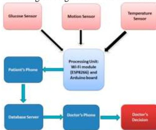
Figure 1 – Hardware block diagram for monitoring the diabetic patient [6]
