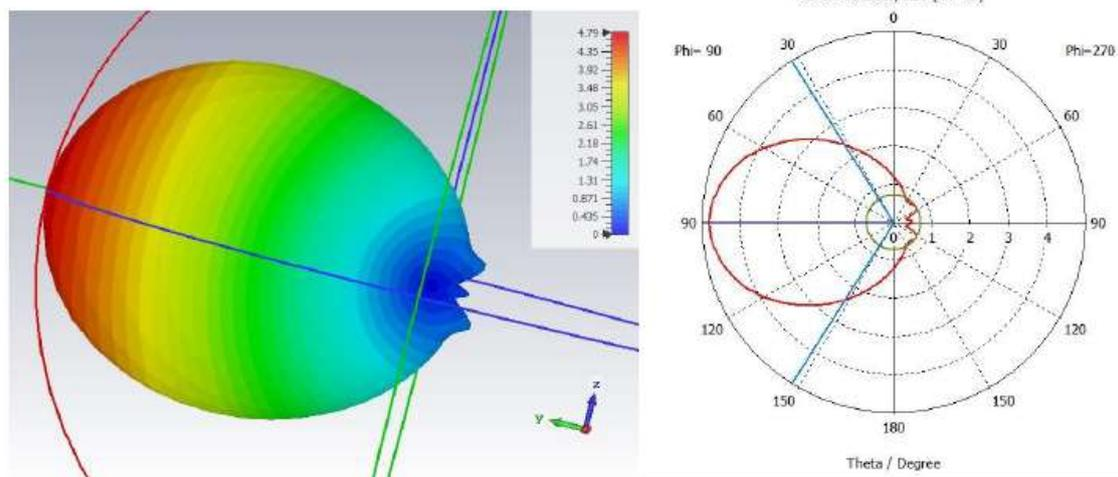
Figure 3 – The directional pattern of a wave with  $f=30\text{ GHz}$  when emitted from the open end of the waveguide
