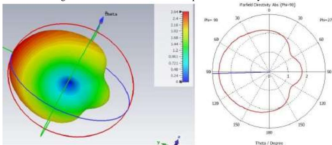
Figure 1 – The directional pattern of a wave with  $f=7,5\text{ GHz}$  when emitted from the open end of the waveguide
