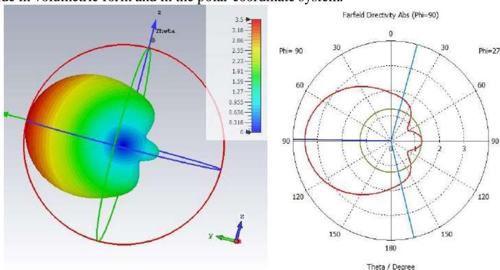
Figure 2 – The directional pattern of a wave with  $f=15\text{ GHz}$  when emitted from the open end of the waveguide
