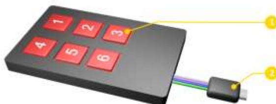
Figure 2 – 3D view of the proposed braille keyboard for smartphone
