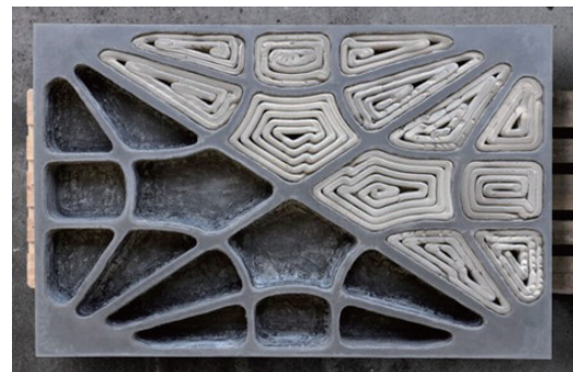
Figure 5. Foam 3D printing inside concrete construction [9]
