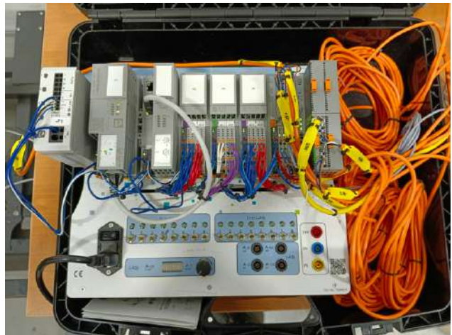
Figure 4. Controller and input/output node of the stand
