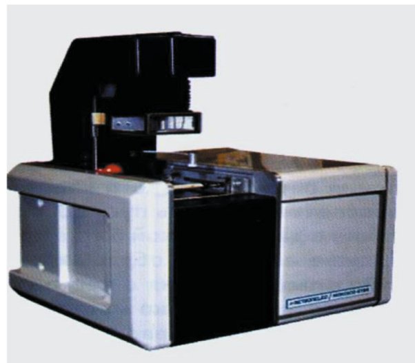
Fig. 13. Menisco ST88 tester for solderability control.
