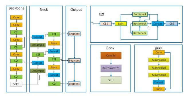
Figure 1. YOLOv8 network model structure diagram
