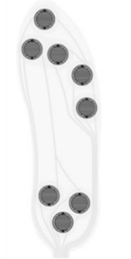
Figure 1. Distribution of insole pressure sensor placement
