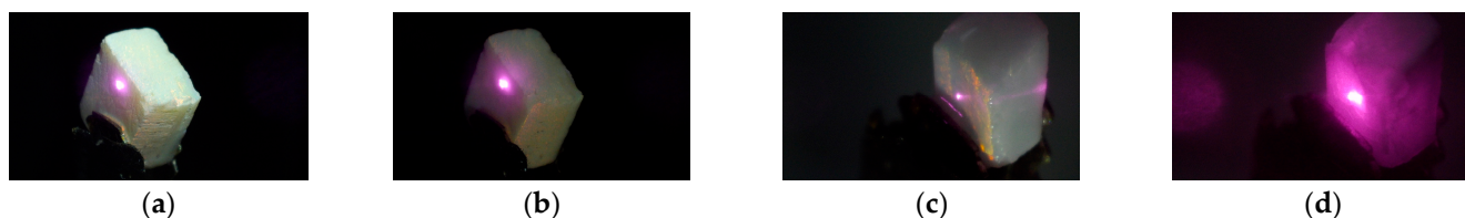
Figure 6. Images of opal matrix (sample #4) under illumination with an IR laser. The area illuminated by the laser does not show upconversion luminescence. The orchid color is the scattered light of the laser detected by the camera. The images from (a) to (d) differ in the area of laser illumination and the white light source.
