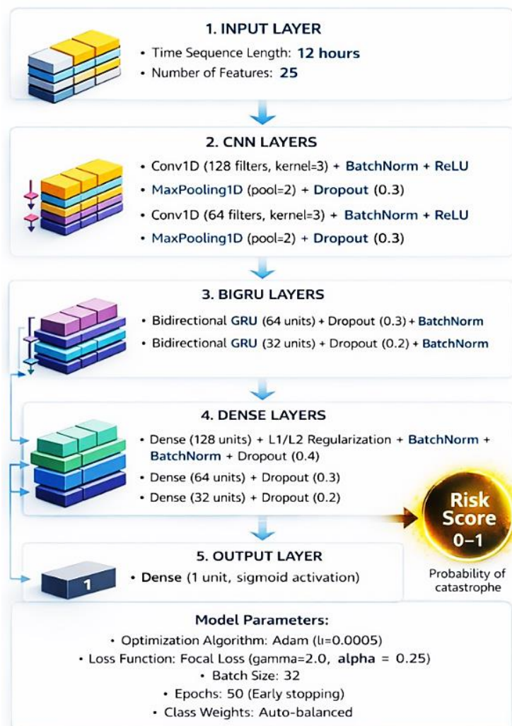
Fig. 1. Architecture of the proposed CNN-BiGRU framework for dam failure risk early warning, illustrating convolutional temporal feature extraction, bidirectional recurrent sequence modeling, and probabilistic risk estimation.
