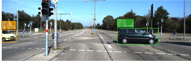
Figure 3. Feature-level Fusion obstacle detection
