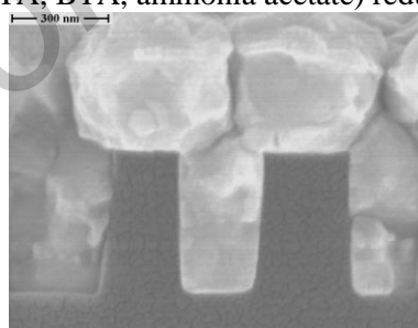
Fig. 5. SEM image of trenches filled from ammoniate solution with PEG-1500 at room temperature
